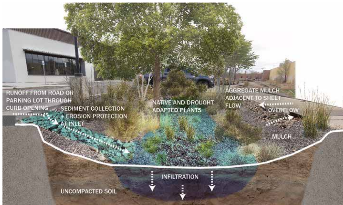
Stormwater harvesting basin schematic
