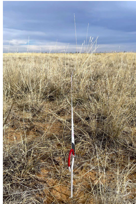
Figure 5. A tape measure has been staked to the ground and unspooled in a straight line.
