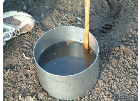
Figure 2. An infiltration test in progress.
