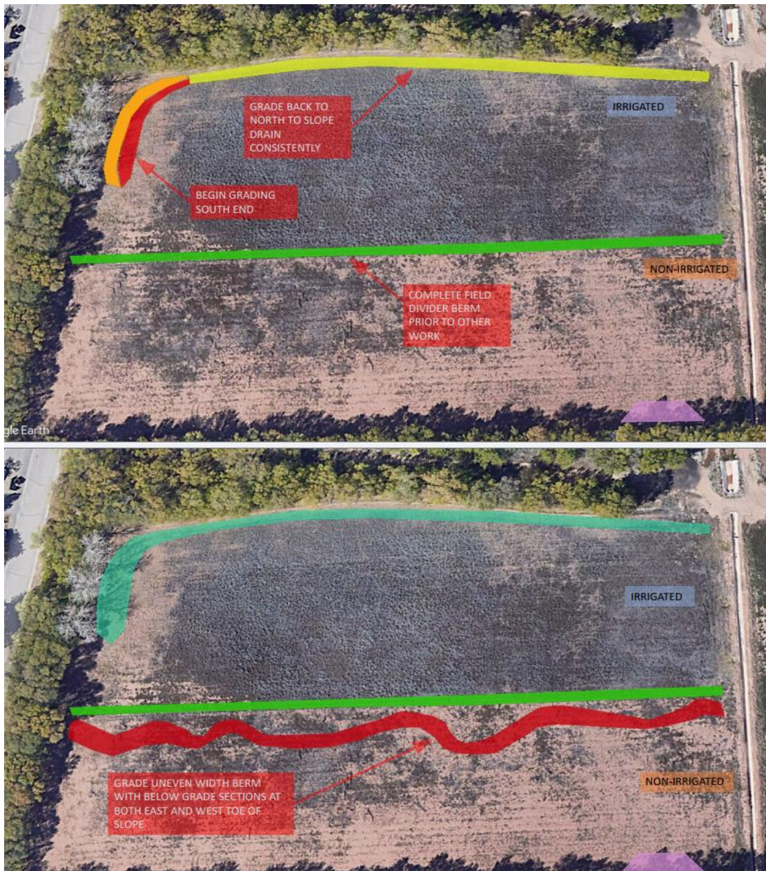
Figure 4. Design-plan schematic for field 4A developed by RGR and CSWCD. Top photo shows first phase of implementation, followed by the second stage in the bottom photo. North direction is approximately to the right of figure.
